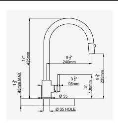
The hole centre for this product should be a minimum distance of 70mm from the wall.
