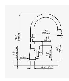
Single flow spout. The hole centre for this product should be a minimum distance of 35mm from the wall.
