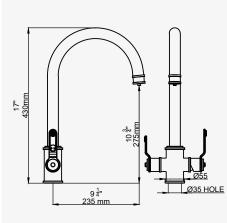
With textured lever handles. The hole centre for this product should be a minimum distance of 80mm from the wall.
