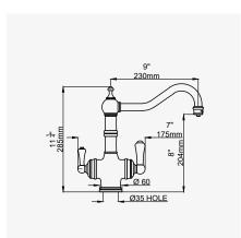
The hole centre for this product should be a minimum distance of 70mm from the wall.
