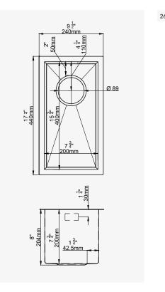
Fully insulated (bottom and sides). 9mm sink base radius for easy cleaning. Resistant to rust and corrosion.
