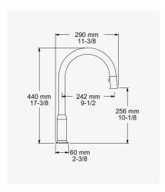
The hole centre for this product should be a minimum distance of 50mm from the wall.
