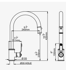
With textured lever handle. The hole centre for this product should be a minimum distance of 90mm from the wall.
